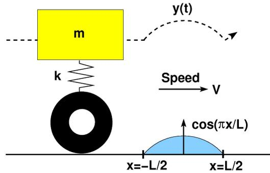
The figure suggests that a crude model of the vertical motion  $y(t)$  of a car encountering the speed bump with speed  $V$  is given by:
