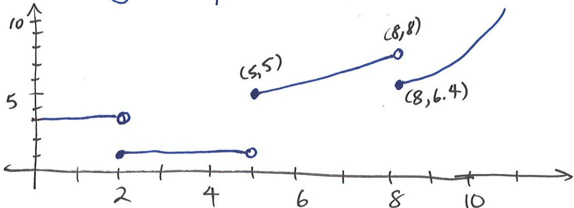
$$f(t) = 3(1 - u_2(t)) + 1(u_2(t) - u_5(t)) \quad * \text{USING PREV. EG.} \\ + t(u_5(t) - u_8(t)) + \frac{t^2}{10}(u_8(t))$$
